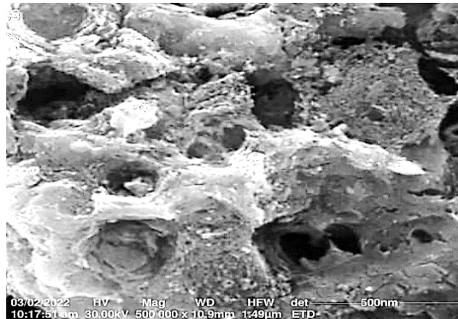
Figure 4: SEM micrograph of VDZnCl 2 adsorbent
